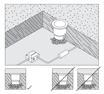
3. Optionally the distribution box (item no. 55380) can be used to connect up to 6 luminaires in the ground to the supply line installed by the customer. After installation, all electric cables are sealed in the distribution box with the supplied cast resin.
