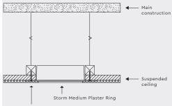
Make sure the Storm Medium Plaster Ring is securely fasten to the reinforcement.
