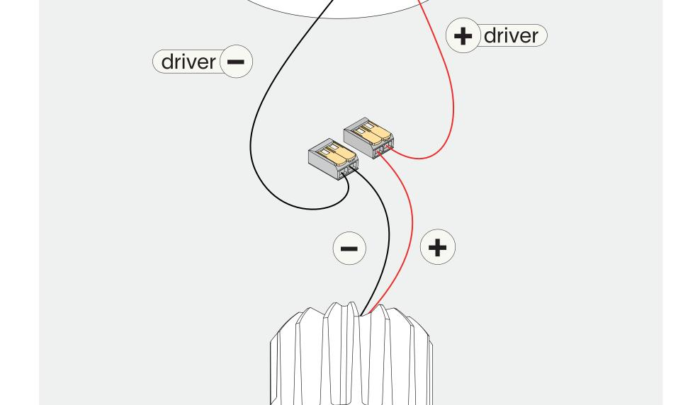
connect the wires with wago connectors
