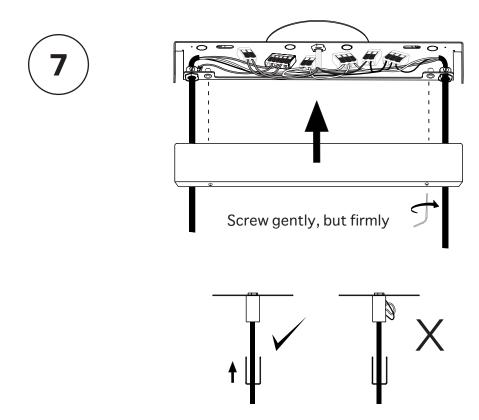
Ensure no wires are clipped or pinched during this operation.
