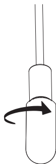
Screw in globe gently until it is tight. Do not force the globe.
