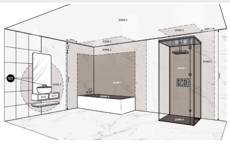
The following information is a guide to help you understand what fittings can be placed in a bathroom. This is not an installation guide and reference should be made to the IEE Wiring Regulations (17th Edition) or a qualified electrician.
